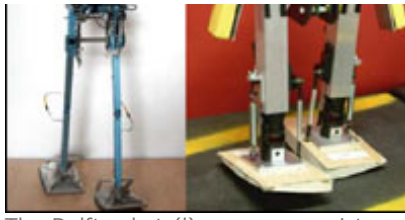
The Delft robot (l) uses gas canisters; MIT's (r) is nicknamed the Toddler
